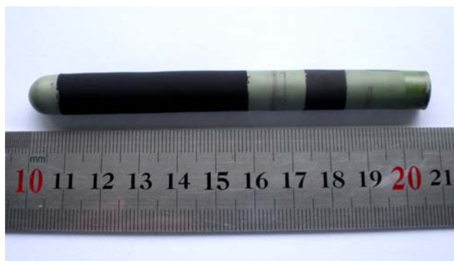
Fig. 3 An anode-supported tubular SOFC with the length of 10.8 cm
